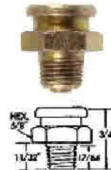
1/8" NPT Pipe Thread Standard Button Head Fitting Part No. 83-B-212
