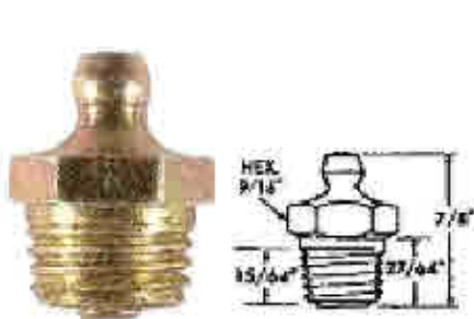
1/4" Pipe Thread Straight / Up to 10,000 PSI Part No. 83-414
